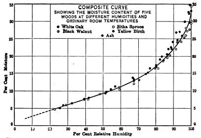
Fig. 101.—Composite curve of moisture content of five woods at different humidities and ordinary room temperature.
